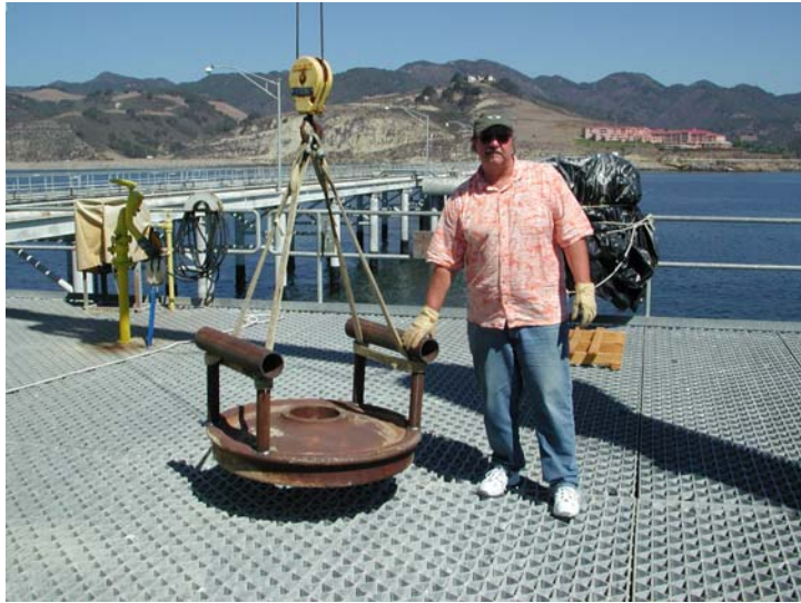
Figure 3. Railroad wheel used to anchor the sensor array.
