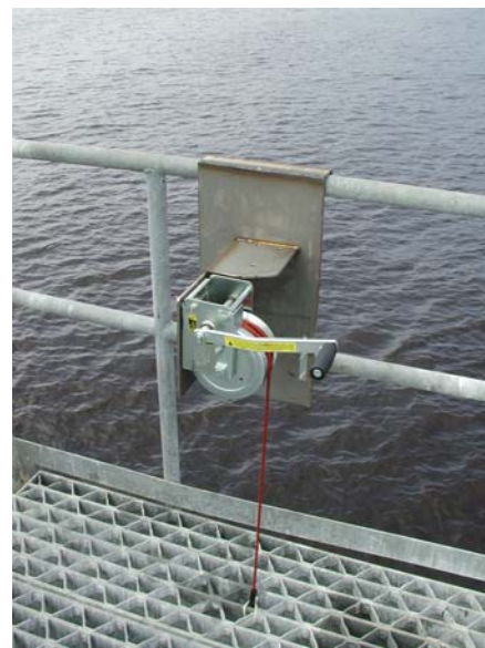
Figure 4. Sensor array tensioning winch.
