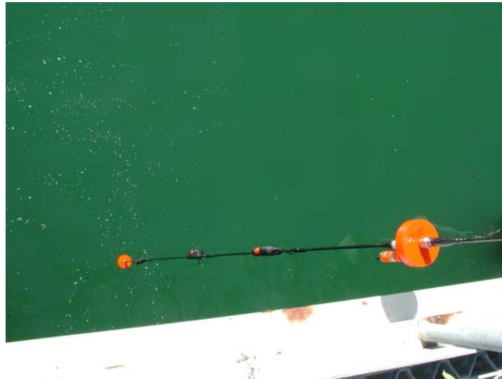
Figure 5. Instrument array suspended above water off the pier showing locations of sensors at five depths.
